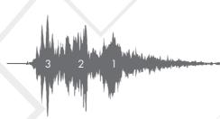
This waveform represents the exact same words, but affected by reverberation. You can clearly see how their shape has changed and how the separation of the words is now blurred – software cuts the "tail" of the reverberation digitally, but the speech clarity is still heavily degraded.
