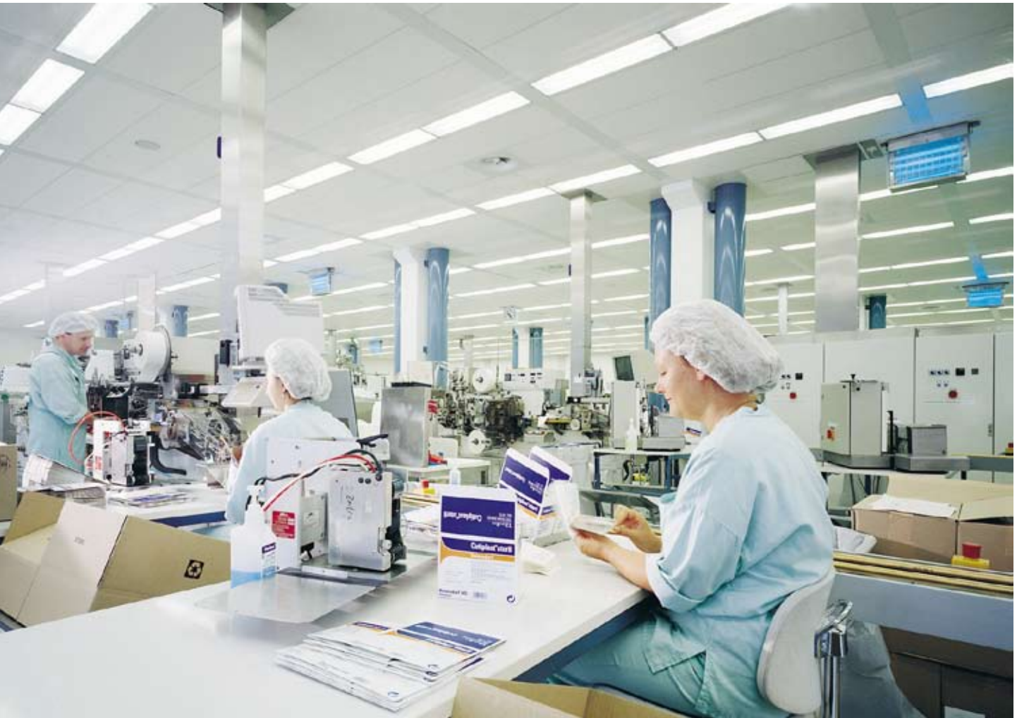
An acoustic wall to wall ceiling decreases the sound spreading from production equipment, creating better working conditions at adjacent stations.
