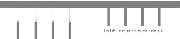
Solo Baffle/hook gives flexibility in level and position.
